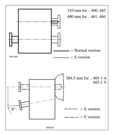
The cast transmission housings are extremely torsionally rigid and, with the exception of the BW 461, are made from a light metal alloy which is almost totally resistant to salt water. The BW 461 transmission housing is made from gray-cast iron. The machined surfaces and tapped holes required for attaching the transmission mountings and the bell housing are included as standard.
