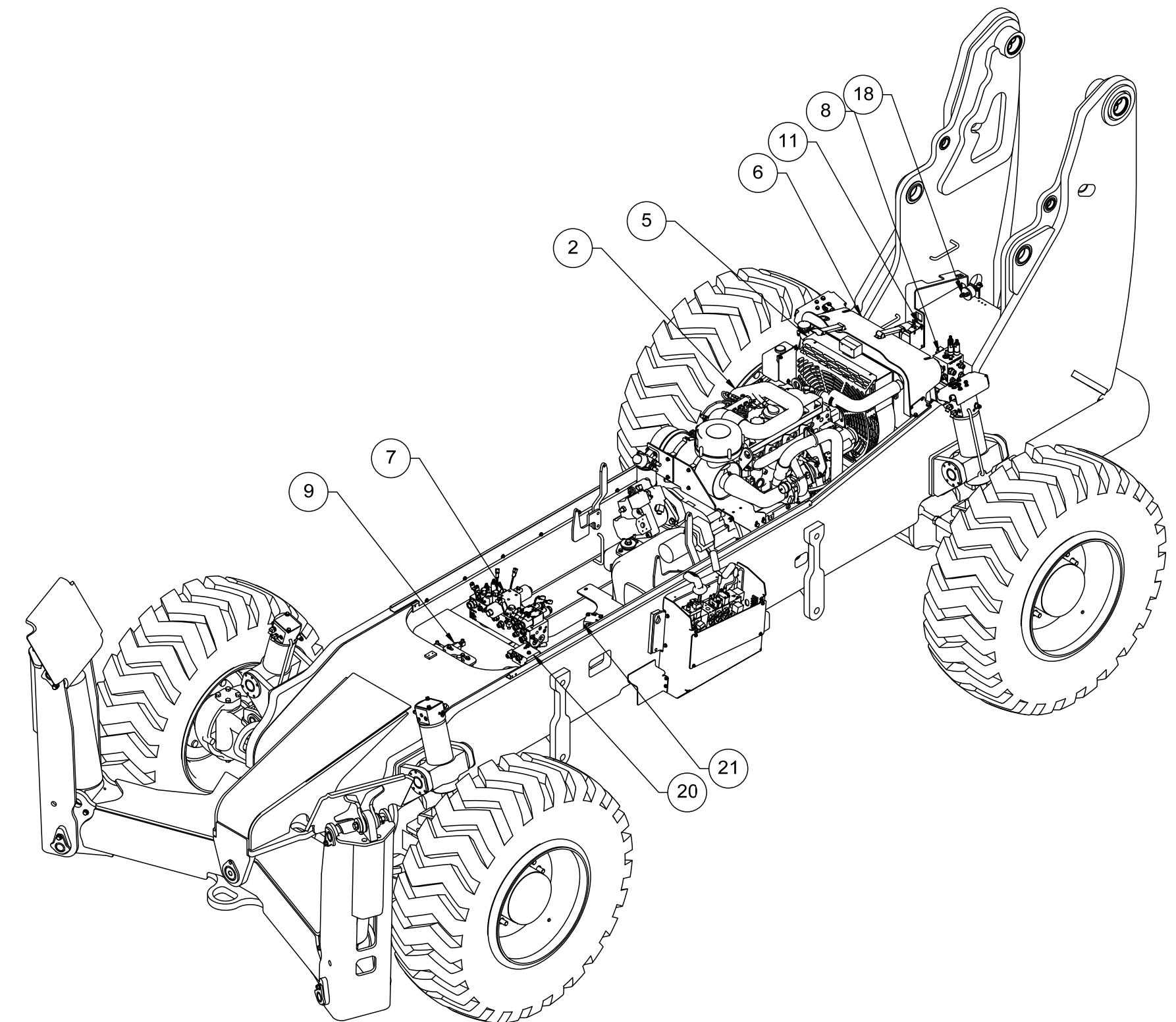
Figure 2-3. Chassis Assembly – Engine (Sheet 1 of 5)
