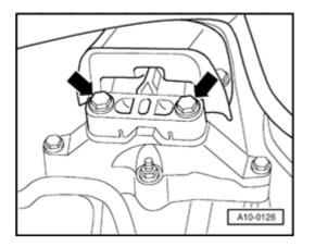
Unbolt transmission side of assembly mounting from top of transmission carrier (arrows).
