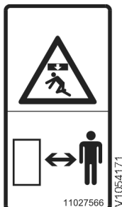
2 WARNING! do not walk under raised attachment (spare part number in usa: 11027566)
