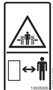
3 WARNING! Risk of crushing at frame joint if machine is steered (Spare part number in USA: 13935000)
