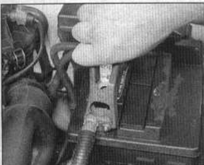
1 Connect one end of the red jump lead to the positive (+) terminal of the flat battery
