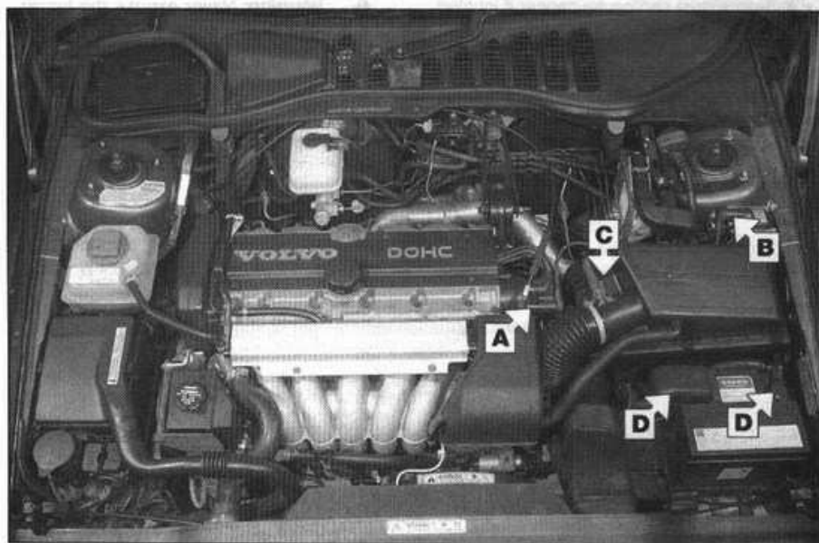
C Check the mass air flow sensor or inlet air temperature sensor wiring connector for security.
