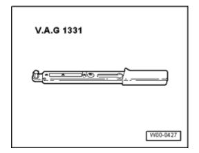
Torque wrench VAG 1331 (or 5 - 50 Nm equivalent)
