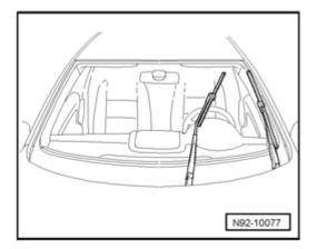
To remove wiper blades, wiper arms must be driven into "service/winter position". The "service/winter position" is activated by operating windshield wiper lever in "touch sweep" position within 10 seconds after switching off ignition  $\Rightarrow$  *Owners Manual*.
