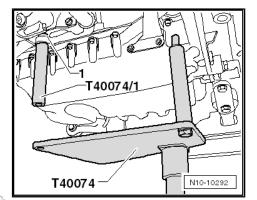
Position engine support -T40074- on engine as shown and retighten adapter -T40074/1- with engine support -T40074--2-.
