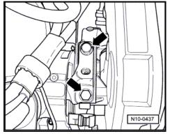
Unbolt gearbox side of assembly mounting from gearbox bracket -arrows- from above.
