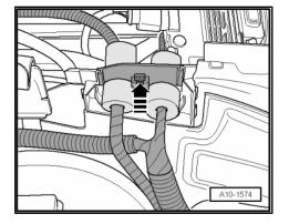
Unscrew cable from alternator at fuse holder -arrow of guarantee of actions of the state of the
