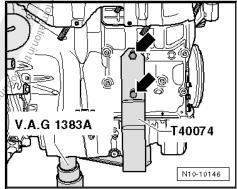
Unbolt engine side of assembly mounting from engine bracket from above -arrows-.
