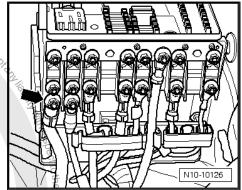
able from whole, is not or in whole, is not or in whole is not or in whole is not one in the search of the search Unscrew earth cable from longitudinal member -arrow-.
