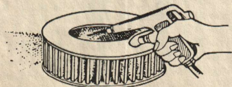
Sometimes the air filter can be cleaned with low pressure compressed air
