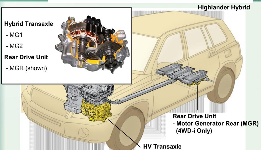
Motor Generator 1 (MG1)Motor Generator 2 (MG2)
