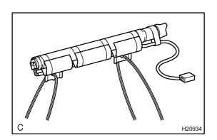
(1) Passing the wire harness through the installation holes as shown in the illustration.
