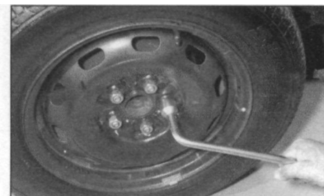
Tighten the wheel nuts securely. Have them checked for tightness using a torque wrench at the earliest opportunity
