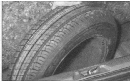
5 Remove the spare wheel from the well in the rear luggage compartment (note that the outer side of the wheel is uppermost)
