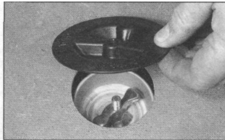
2 Fold back the boot carpet and unscrew the plastic nut from the top of the spare wheel retaining stud
