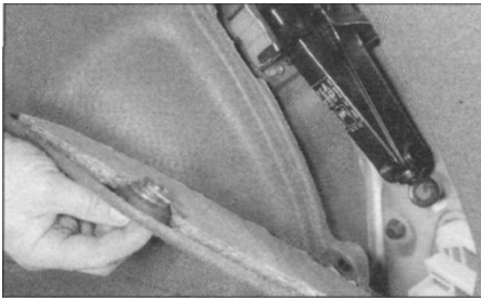
1 The jack is positioned in the right-hand rear of the luggage compartment. The brace is located beneath the jack
