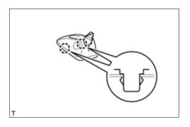
(c) Disengage the 2 claws and remove the amplifier antenna assembly.
