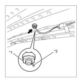
(b) Place the amplifier antenna cord in the amplifier antenna cutout.
