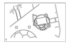
(a) Disengage the 3 claws and remove the front No. 2 speaker assembly from the No. 1 instrument speaker panel sub-assembly.
