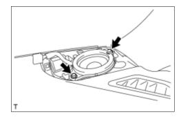
(b) Remove the 2 bolts and the front No. 3 speaker assembly.
