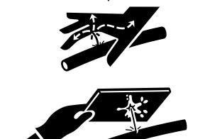
Pressure is maintained in the hydraulic circuit long after the engine has been shut down.
