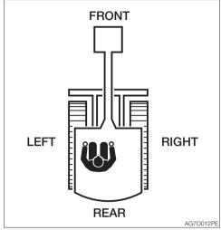
This manual refers the front, rear, left and right of the machine as seen when sitting in the operator's seat with the dozer blade visible to the front.
