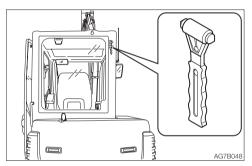
An emergency hammer is installed to be used to escape from the cab in an emergency. When escaping, break the windows with the hammer.
