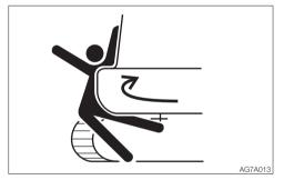
Never put your hands, feet or other parts of your body between the upperstructure and the undercarriage or tracks, between the machine body and working equipment, or between a cylinder and moving part. The sizes of these gaps change when the machine moves, and a person can suffer severe injury or death.
