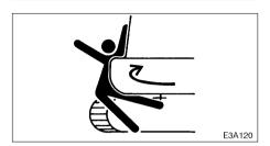
Never put your hands, feet or other parts of your body between the upperstructure and the undercarriage or tracks, between the machine body and working equipment, or between a cylinder and moving part. The size of these gaps change when the machine moves and if caught a person can suffer severe injury or death.
