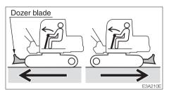
Before operating the travel levers, check to make sure that the dozer blade is to the front of the operator's seat. BE AWARE that when the dozer blade is to the rear of the operator's seat, the travel levers operate in the opposite direction to when the dozer blade is in the front.
