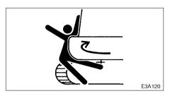
Never put your hands, feet or other parts of your body between the upperstructure and the undercarriage or tracks, between the machine body and working equipment, or between a cylinder and moving part. The size of these gaps change when the machine moves and if caught a person can suffer severe injury or death.
