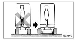
Always operate the machine with the crawler width at the maximum to increase machine stability. The smaller the crawler width, the greater the possibility the machine can tip over. If it is absolutely necessary to operate the machine with a narrow crawler width, do so with great care.
