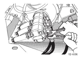
3. After installation of hydraulic hoses or steel pipes, apply the maximum working pressure 5 or 6 times and confirm that there is no leakage.
