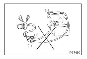
When applying a voltage to a part for inspection purposes, check that the (+) and (-) cables are connected properly then gradually increase the voltage from zero. Do not exceed the specified voltage.
