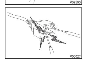
• When using a multimeter to check continuity, do not allow the test probes to touch the wrong terminals.
