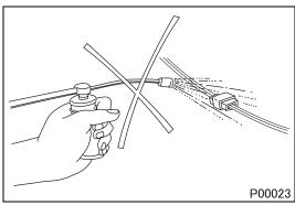
Before washing the vehicle, cover all electrical parts to keep them dry. (Use plastic sheets or the like.) Keep water away from harness connectors and sensors and immediately wipe off any water that gets on them.
