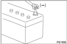
Before working on the electrical system, disconnect the battery
