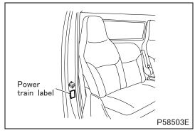
The power train label, located on the passenger door B-pillar, indicates the vehicle model, chassis number and the serial numbers of the vehicle's powertrain components.
