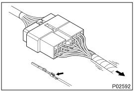
• Check for wires that have separated from their terminals due to pulling of the harness.
