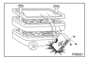
Carefully handle sensors, relays, and other items that are sensitive to shock and heat. Do not remove or paint the cover of any control unit.
