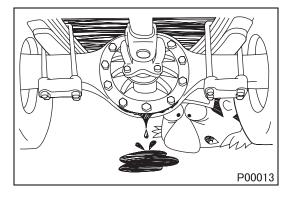
• Inspect for fluid leaks before washing the vehicle. Signs of fluid leaks may go unnoticed on a freshly-washed vehicle.
