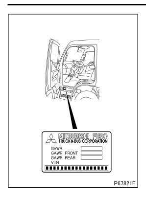
The vehicle identification number is punch-marked on the plate attached inside the driver's door, as shown in the illustration.
