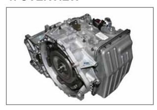
Engine power reaches the transaxle via a torque converter with integral converter lock-up clutch. The six forward gears and one reverse gear are obtained from a single planetary set, followed by a double planetary set. This type of gear-set arrangement is commonly known as Lepelletier type gear-set.
