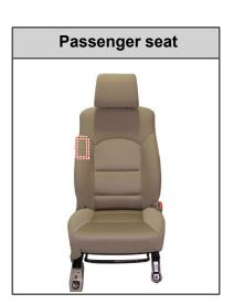
The side air bags are installed in the outer sides of the driver's and passenger's seats to minimize occupants' side injuries in case of a side impact.
