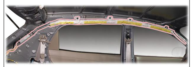
The curtain air bags, which are part of the side air bag system, are installed in both roof side rails.
