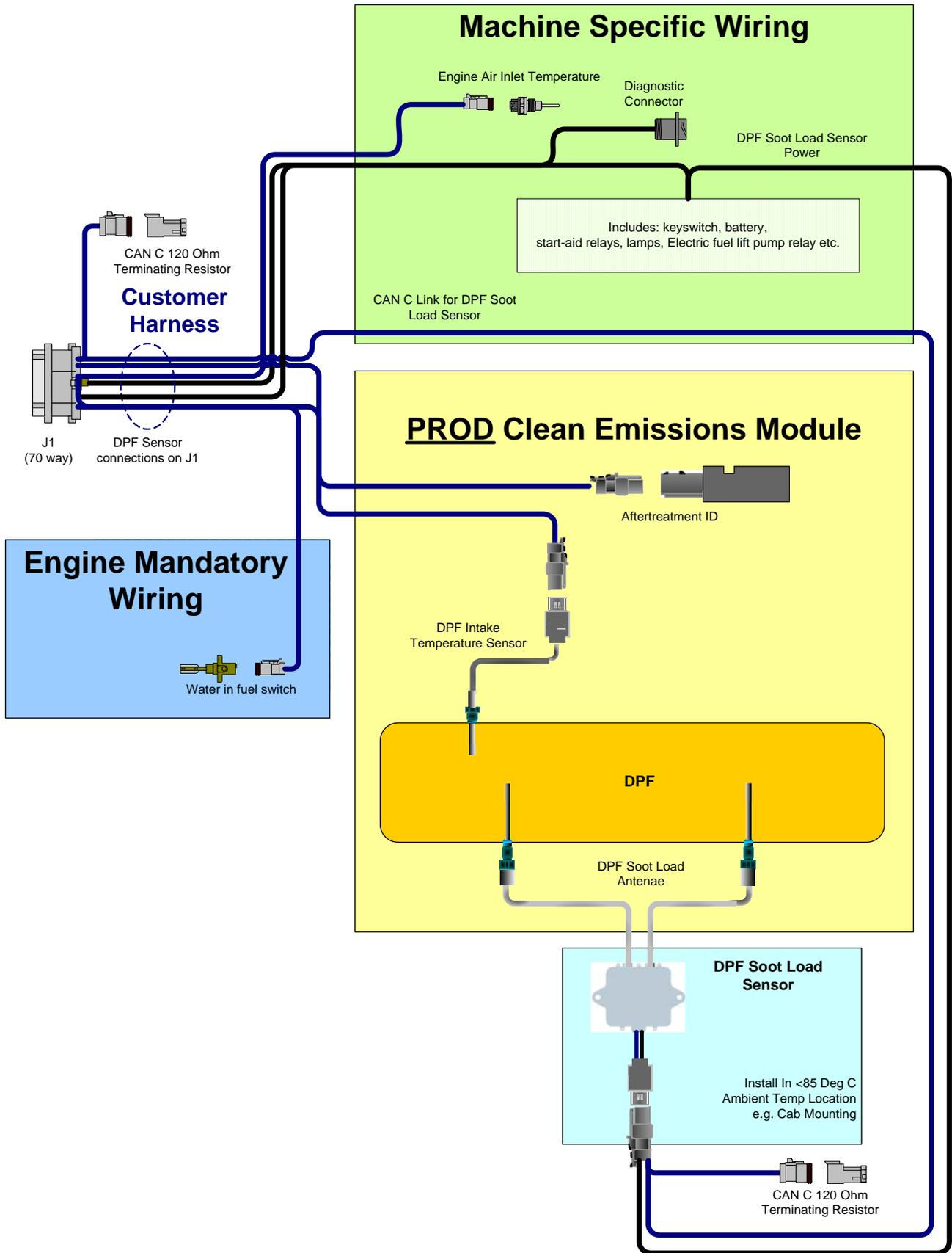
2.3.3 1206E-E66TA Factory Installed Wiring and Components
