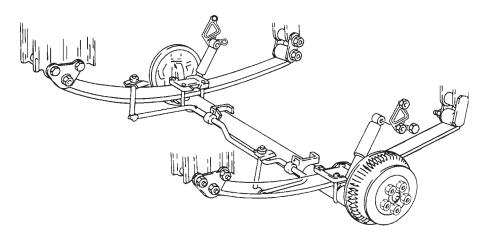
In both suspension designs, the leaf springs are mounted to the frame rails, providing added strength and durability. Wide-design long leaf springs minimize movement during lateral maneuvers, improving handling performance. The leaf spring design also provides superior management of cargo loads and towing.
