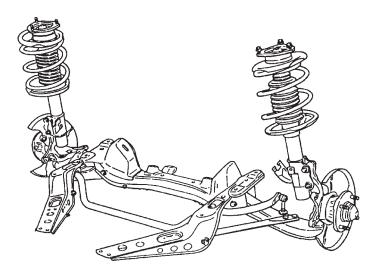
The independent strut front suspension uses a coil spring and a shock strut combined into one unit. The strut is an integral part of the system and provides the suspension upper mounting to the body. A lower control arm supports the suspension at the bottom. Compared to many other suspension designs, strut systems use fewer parts and generally weigh less.
