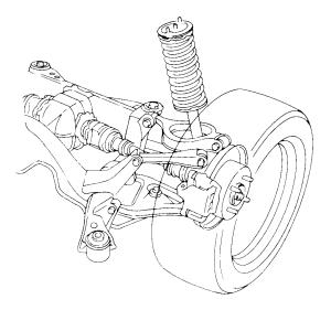
Coil springs are used on the front and rear suspensions of all Nissan sedans and Pathfinder, as well as the Quest front suspension. All 2002 Infiniti vehicles use coil springs in the front and rear suspension systems.
