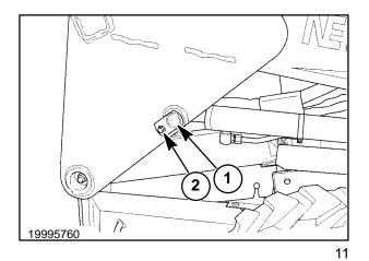
5. Support the cylinders on the fenders, 1, as shown.
