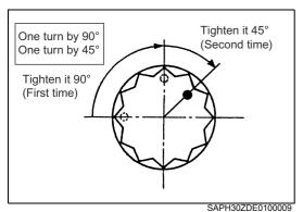
(3)Tightening method after tightening to seating torque Tightening of 90°, 135° (90° once and 45° once) and 180° (90° twice) is available.
