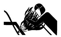
Make sure there is good ventilation. Wear eye protection and protective equipment when welding.
