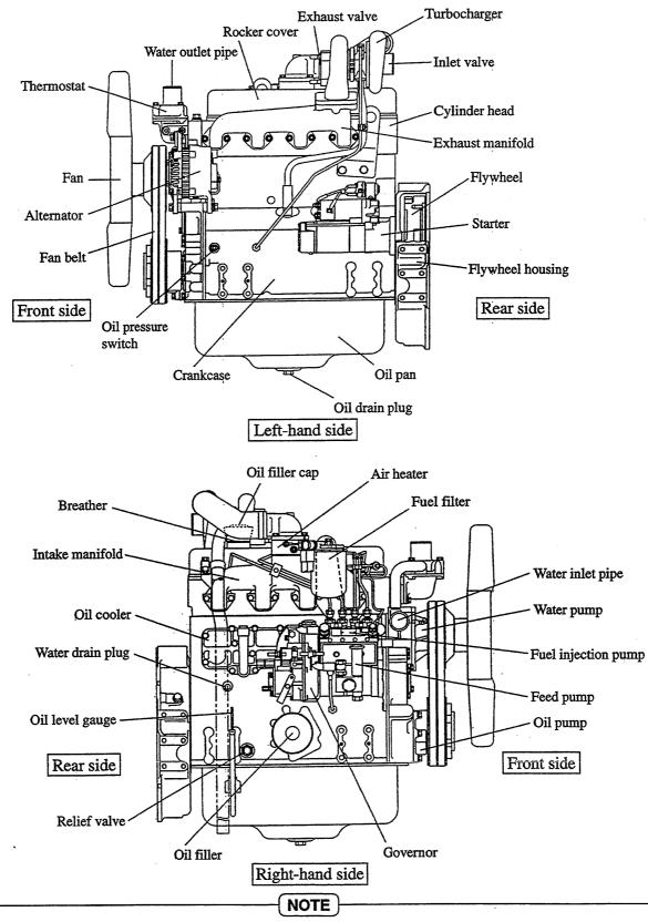
Direction of rotation when viewed from the flywheel side is to the rear left (counterclockwise).
