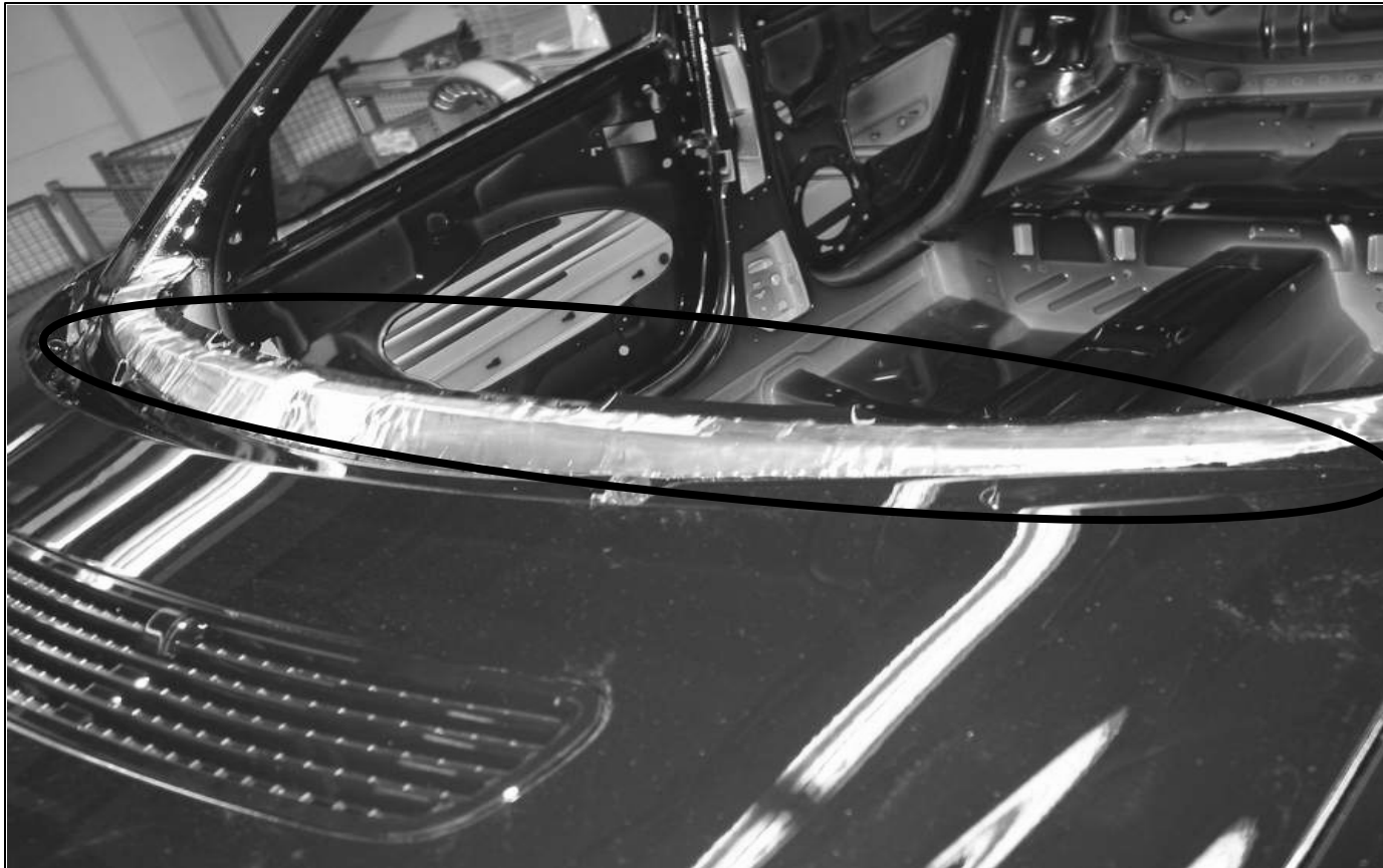
Extra insulation at windshield base
