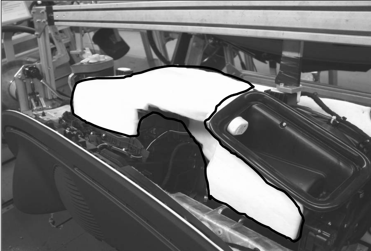
Noise insulation installed around heater box
