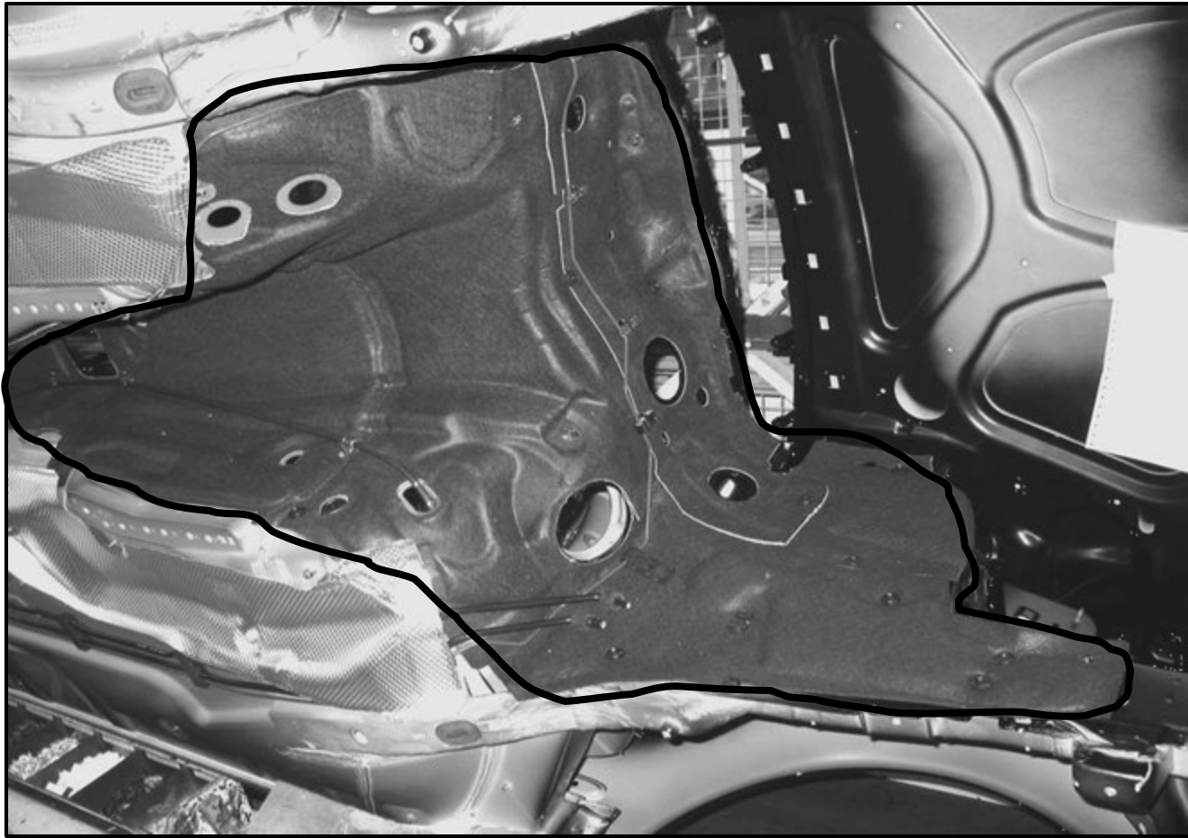
Underbody insulation panel bulkhead and tunnel area
