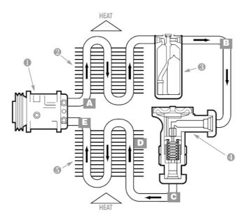
2. Technician A says that at point E in this illustration the refrigerant is high pressure vapor.
