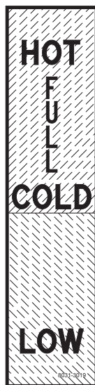
Located on reservoir by pressure fill port Part No. 8031-3019
