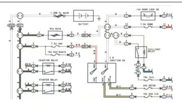
The ground points circuit diagram shows the connections from all major parts to the respective ground points. When troubleshooting a faulty ground point, checking the system circuits which use a common ground may help you identify the problem ground quickly. The relationship between ground points ( $\mathbf{W}$ ,  $\mathbf{W}$ , and  $\mathbf{W}$ , shown below) can also be checked this way.
