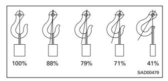
Do not sling a heavy load with one rope alone, but sling with two or more ropes symmetrically wound on to the load
