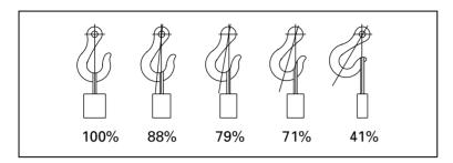
3. Do not sling a heavy load with one rope alone, but sling with two or more ropes symmetrically wound onto the load.
