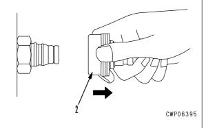
Hold the mouthpiece of the tightening portion and push body (2) in straight until sliding prevention ring (1) contacts contact surface a of the hexagonal portion at the male end.
