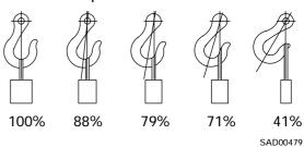
3) Do not sling a heavy load with one rope alone, but sling with two or more ropes symmetrically wound onto the load.
