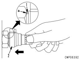
Hold in the condition in Step 1), and turn lever (4) to the right (clockwise).
