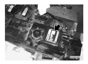
The plate regarding the exhaust emission regulations is applied to the front side of the tappet cover.
