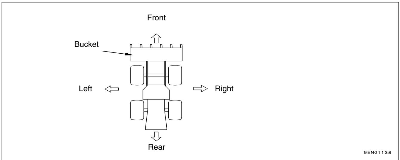
In this manual, the directions of the machine (front, rear, left, right) are determined according to the view from the operator's seat in the direction of travel (front) of the machine.
