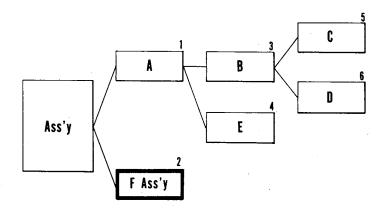
The sequence of the procedural steps is given in arabic numbers on the top right of each block. For example, when it is necessary to remove part D from the assembly, the steps for removal should be  $A \rightarrow B \rightarrow D$ . Or, to remove part E the step is  $A \rightarrow E$ . F Ass'y is an assembly for which the disassembling procedure is described separately. For assembly, the sequence is presented under each section, in the same manner as for disassembly.
