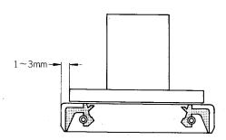
When installed, the oil seal should not be inclined at an angle. Press-fitted angle of an oil seal should not exceed the permissible limit of 0.2 mm/100 mm dia.
