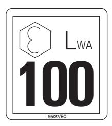
Noise level indicated is the guaranteed value measured by the dynamic test method as specified in the directive 86/662/EEC, as amended by 95/27/EC.
