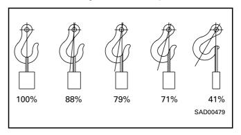
Do not sling a heavy load with one rope alone, but sling with two or more ropes symmetrically wound on to the load.
