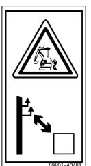
Sign indicates an electrocution hazard if machine is brought too near electric power lines.
