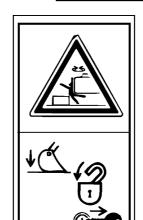
Sign indicates a hazard of being caused or run over by unexpected moving of stopped machine.
