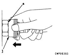
3) Hold in the condition in Steps 1) and 2), and pull out whole body (2) to disconnect it.
