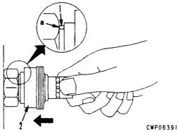
Hold in the condition in Step 1), and push until cover (3) contacts contact surface a of the hexagonal portion at the male end.
