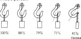
Do not sling a heavy load with one rope alone, but sling with two or more ropes symmetrically wound on to the load.
