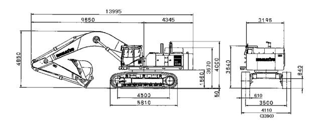
★ The figures in ( ) show the value when the track width is retracted.
