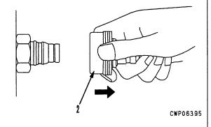
Hold the mouthpiece of the tightening portion and push body (2) in straight until sliding prevention ring (1) contacts contact surface a of the hexagonal portion at the male end.
