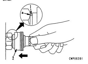
2) Hold in the condition in Step 1), and push until cover (3) contacts contact surface a of the hexagonal portion at the male end.
