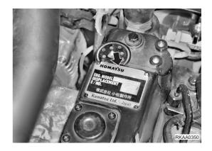
The exhaust gas emission plates are positioned on the upper side of the tappet cover and on the inner right side of the counterweight.
