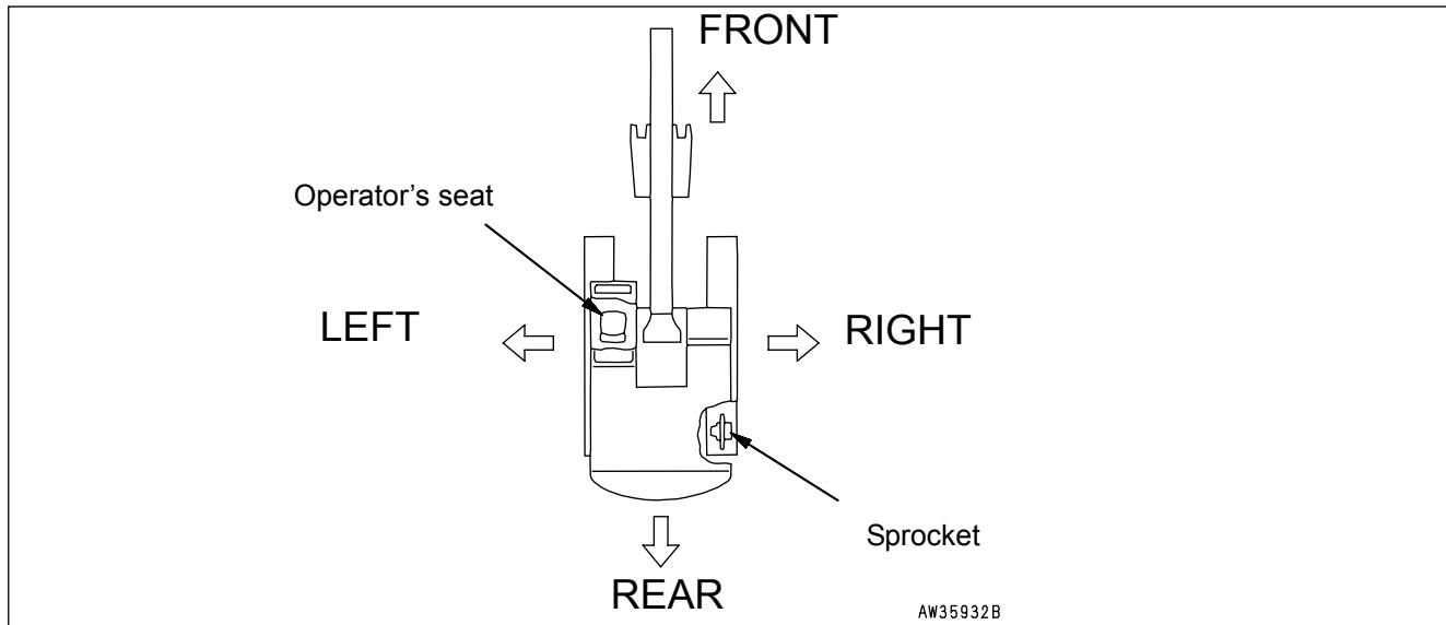
In this manual, the terms front, rear, left, and right refer to the travel direction as seen from the operator's cab when the operator's cab is facing the front and the sprocket is at the rear of the machine.
