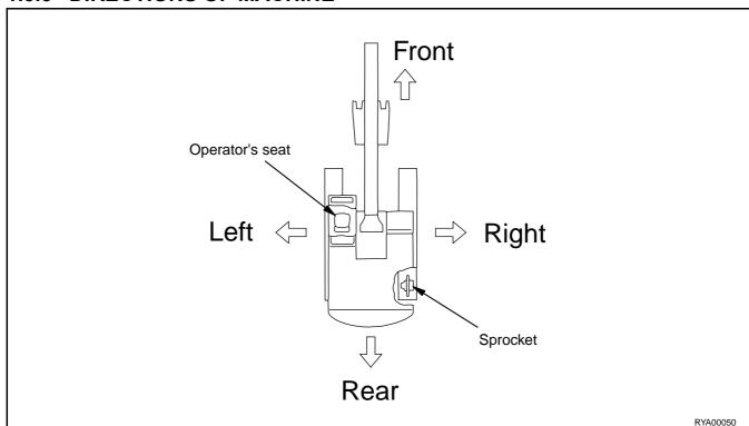
In this manual, the terms front, rear, left, and right refer to the travel direction as seen from the operator's seat when the operator's seat is facing the front and the sprocket is at the rear of the machine.
