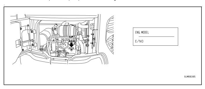
The exhaust gas emission plate is positioned on the radiator chassis.
