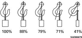
3) Do not sling a heavy load with one rope alone, but sling with two or more ropes symmetrically wound onto the load.
