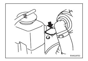
The exhaust gas emission plate is applied on the top of the engine cylinder head cover.
