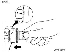
2) Hold in the condition in Step 1), and push until cover (3) contacts contact surface a of the hexagonal portion at the male end.
