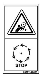
Sign indicates a hazard of rotating parts, such as belt.
