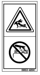
Sign indicates a burn hazard from spurting hot water or oil if radiator or hydraulic tank is uncapped while hot.
