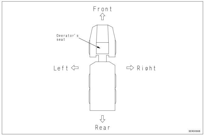
In this manual, the directions of the machine (front, rear, left, right) are determined according to the view from the operator's seat in the direction of travel (front) of the machine.
